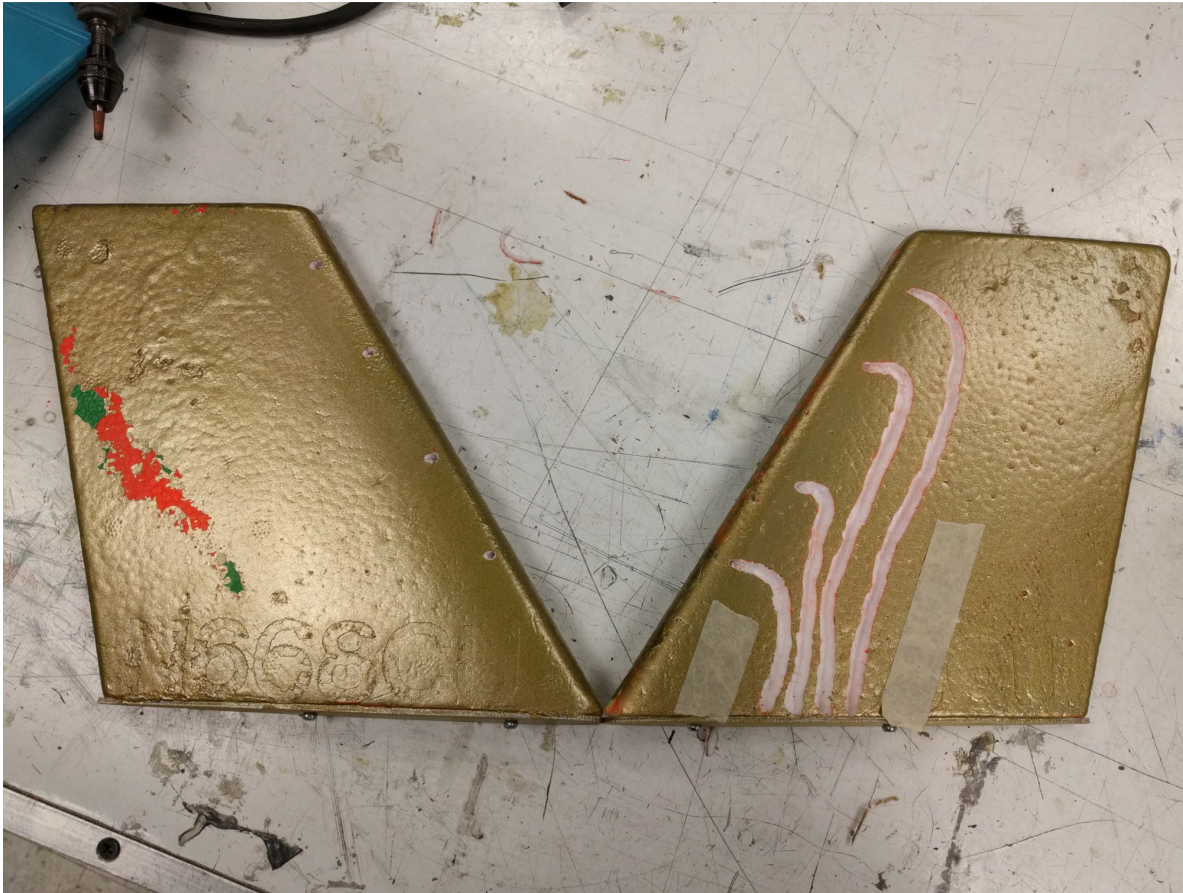
Figure 3.23: Early work on the sideplates. Note the channels created for routing tubing from the physical port locations to the sealed circuit boards installed in the wings.
