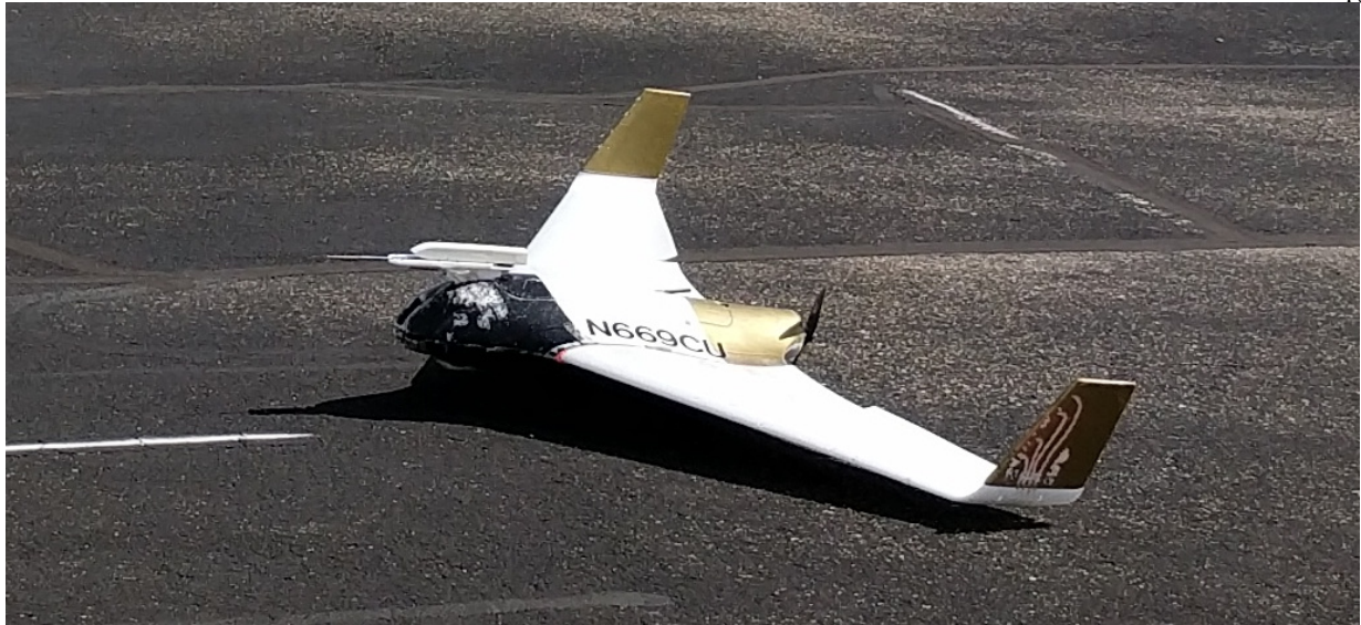
Figure 2.1: Aeroprobe MHP mounted on the X-8 Skywalker UAS.
