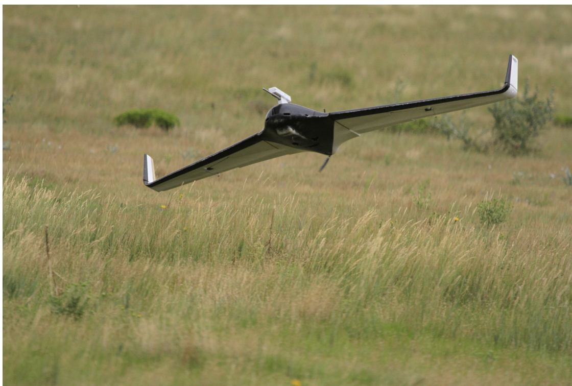
Figure 1.2: Photo of the Skywalker UAS coming in to land. Note the exposed probe above the nose. Photo credit: Joanie Wiesman, CU Boulder.
